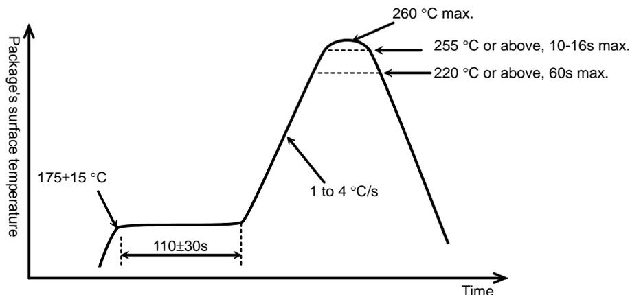
Figure 1: Infrared reflow, air reflow temperature profile
